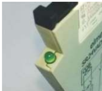
Relay Coil Energised Indication
